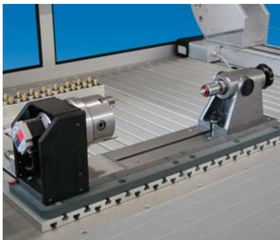
Rotary axis with three-jaw chuck (left) and tailstock unit with sleeve (right)
