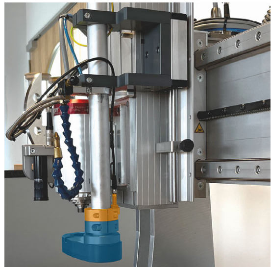
FIG. 24 ELECTRONICALLY MONITORED SUCTION SHOE
