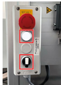
FIG. 26 CONTROL ELEMENT WITH EMERGENCY STOP AND ACKNOWLEDGMENT BUTTON
