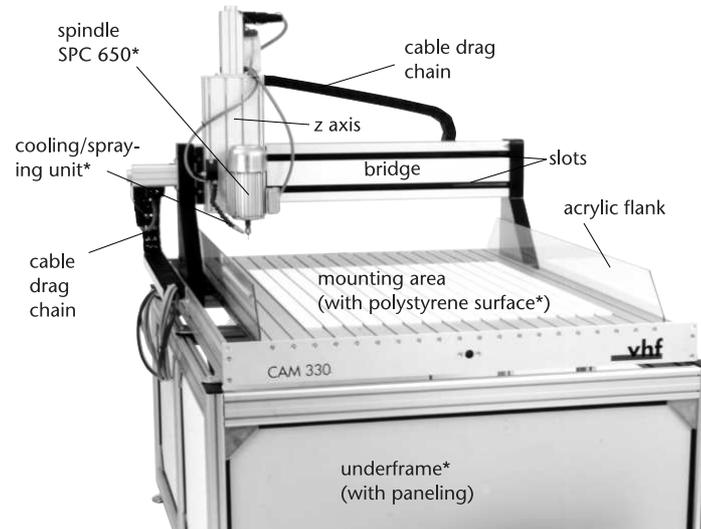
*[Illustration: Components of a CAM 330 Classic (the components marked \* are not included in the delivery of a basic system)]*
