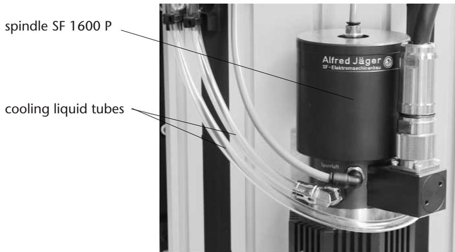
*[Illustration: Flexible tubes for cooling liquids on SF 1600 P]*
