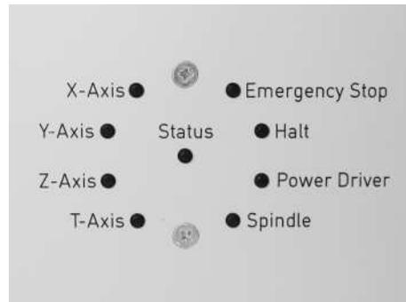
*[Illustration: LEDs on the front side of the controller CNC 580]*
