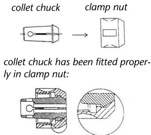
[Illustration: Inserting the collet chuck]
