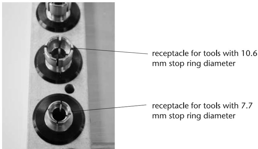
*[Illustration: Receptacles for tools with different stopper ring diameters]*
