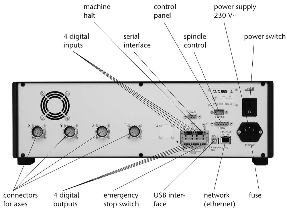
[Illustration: Reverse side of the controller CNC 580]
