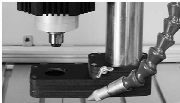
*[Illustration: Dust extraction unit, here with cooling/spraying unit in the foreground]*
