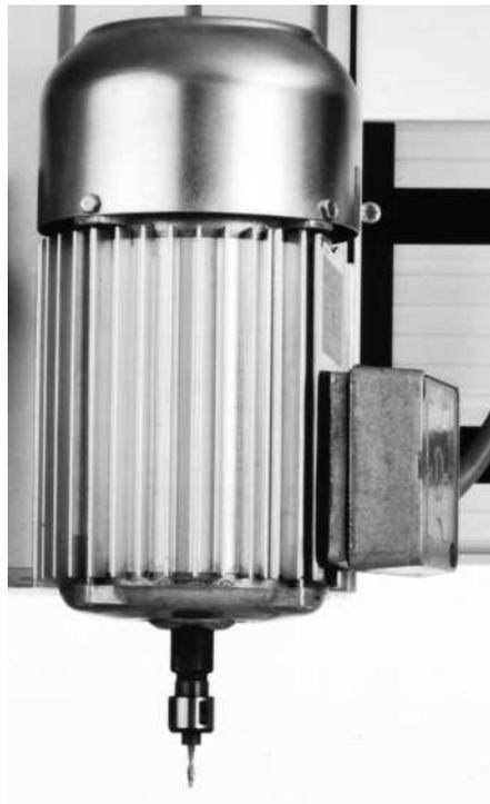
*[Illustration: Three phase rotary current spindle SPC 650 mounted on z-axis]*
