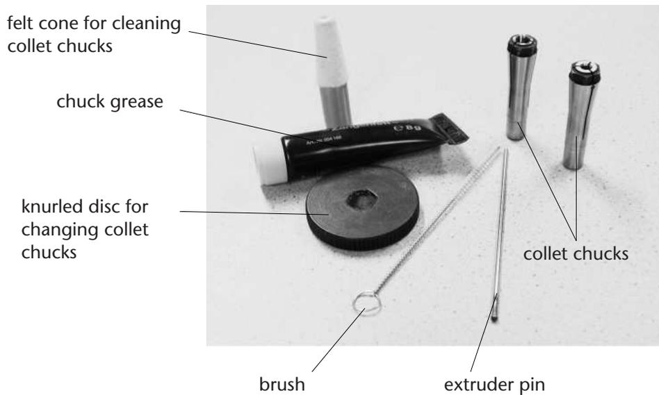
*[Illustration: Service set for pneumatic spindles]*
