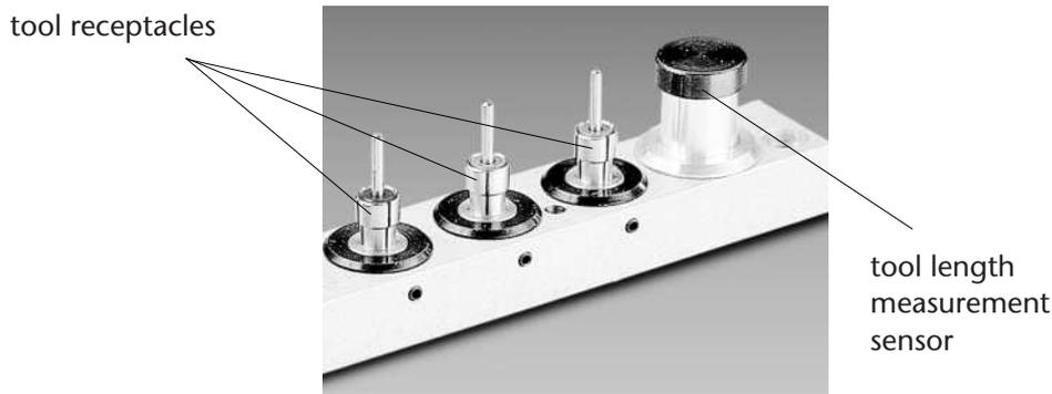
*[Illustration: Tool changing station with height measurement sensor]*
