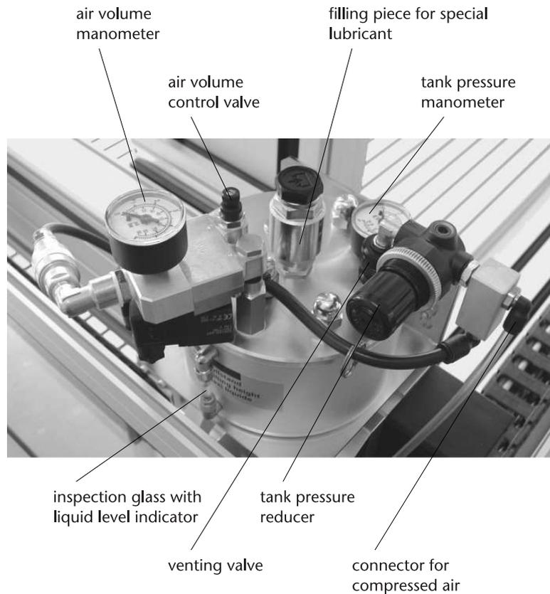
*[Illustration: pressure tank with controls and instruments of the minimum quantity lubrication unit]*
