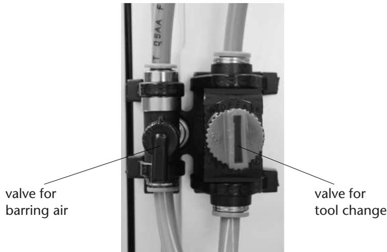
*[Illustration: Pneumatic valves on the z-axis – here in "open" position]*
