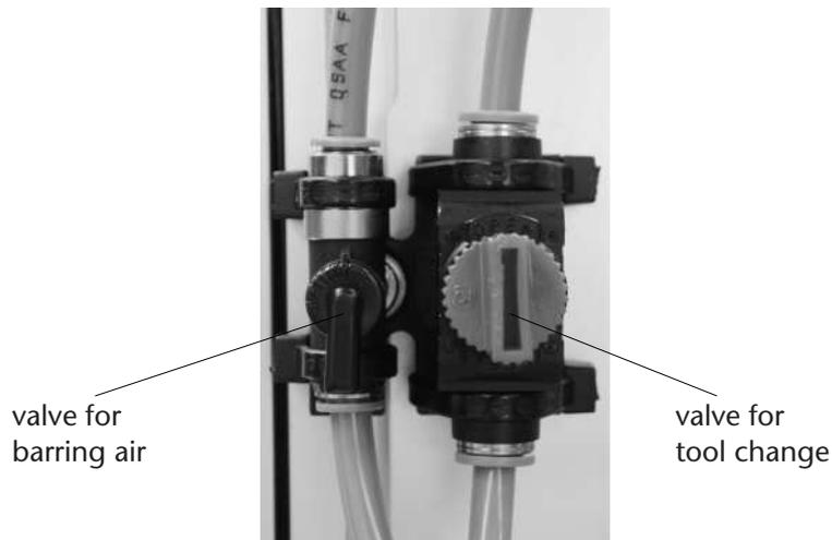
*[Illustration: Pneumatic valves on the z-axis must be in the "open"-position when working with the automatic tool change]*
