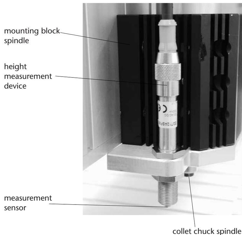
*[Illustration: Height measurement unit, mounted beside the spindle]*
