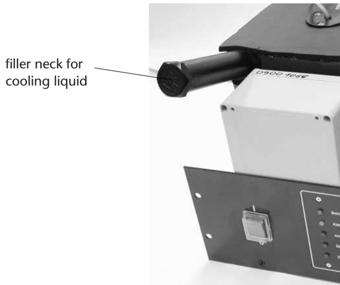
*[Illustration: Filling in of cooling liquid]*
