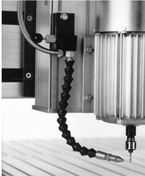
*[Illustration: Cooling and spraying unit]*
