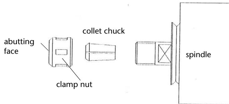
*[Illustration: Inserting the collet chuck]*
