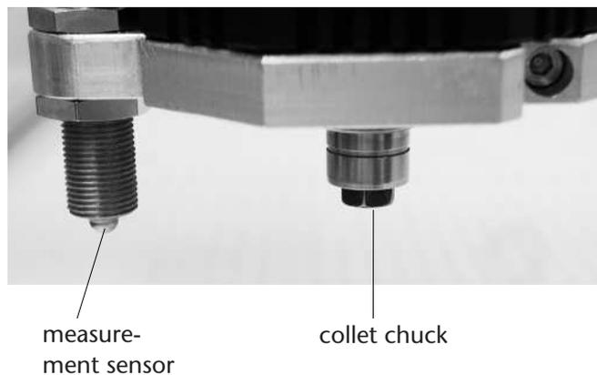
*[Illustration: The pin of the measurement sensor must be some way below the collet chuck]*
