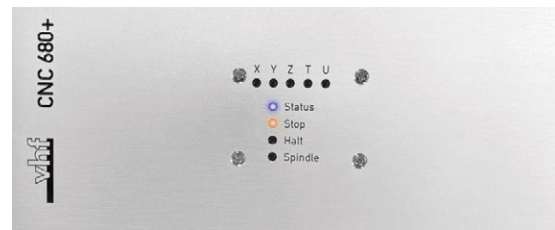
FIG. 19 ORANGE LED EMERGENCY STOP
