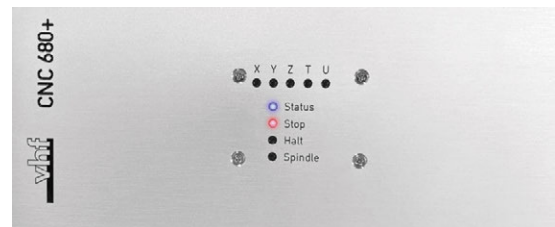
FIG. 20 RED LED EMERGENCY STOP
