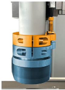
FIG. 16 ELECTRONICALLY MONITORED SUCTION SHOE
