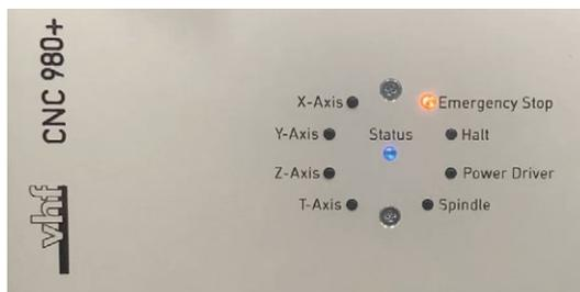
FIG. 45 ORANGE LED EMERGENCY STOP
