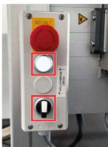
FIG. 27 CONTROL ELEMENT WITH EMERGENCY STOP AND ACKNOWLEDGMENT BUTTON
