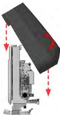
FIG. 76 PLACING THE HOOD
